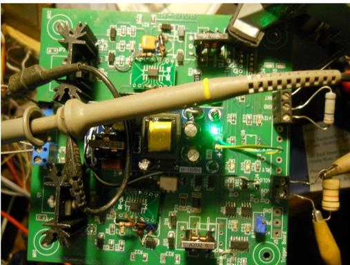
The two common mode chokes are used as transformers to provide two isolated 12V drive power supplies for the two SCR gates, or in this case, MOSFET gates, using an IRS2453 self-oscillating Hi-Lo dual gate driver, at 100 kHz and two dual NMOS devices. They use SI8261 opto-emulated gate drivers, controlled by the PIC16F1778, which provides a 20 kHz PWM. The main 12VDC is supplied with a 12V 1A switching supply (about \$3 from Banggood).
