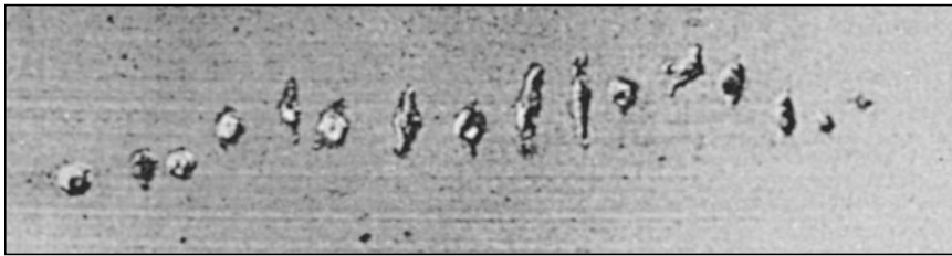
Figure 23 — Electrical pits are another indication of bearing currents. If left unchecked, this will eventually result in fluting.
