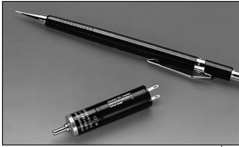
Figure 12 — Typical of miniature motors, this dc motor is 0.511 in. in diam and 1.24 in. long. It has an output power rating of 2.5 W at 8,000 rpm. The construction consists of Neodymium magnets, precious metal brushes, and a moving-coil rotor that uses a Rhombic-wound winding for maximum winding density. A matching 0.511-in. planetary gearhead offers five ratios from 4:1 to 1,118:1 and torque capability to 0.35 Nm continuous and 0.53 Nm intermittent.
