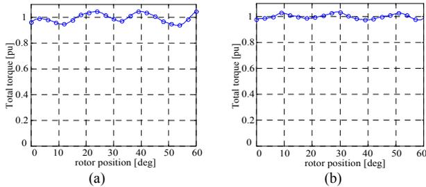
Fig. 10. Total torque of the non-slotted internal rotor type machine (a) without and (b) with skewed rotor magnets
