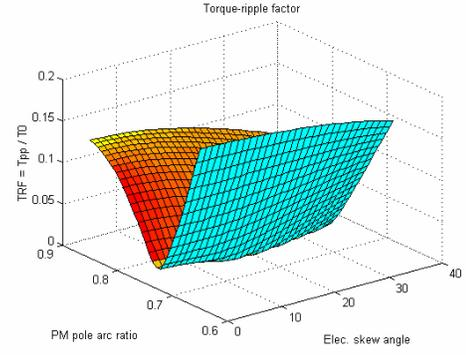
Fig. 4. Torque Ripple Factor of the slotless TORUS machine with rectangular shaped winding as a function of pole arc and magnet skew angle
