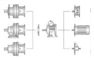
♦ The DARALI® DISCO VARIATOR is a mechanical speed variator that is inherently explosion-proof. Just add an explosion-proof motor, and you can have the adjustable speed versatility in a hazardous environment.
