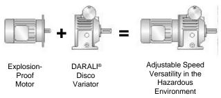
◆ Since motor is always running at full speed, you will always get high torque and maximum cooling effect even at low output rpm.
