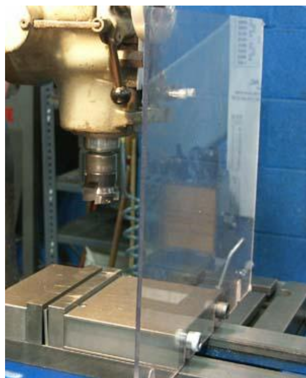
Figure 2. A chip guard protects operators from contact with hot chips.
